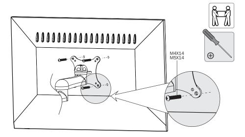
Lift the display and match the holes on your display with the holes on the mount. Secure your display to the mount by tightening screws
